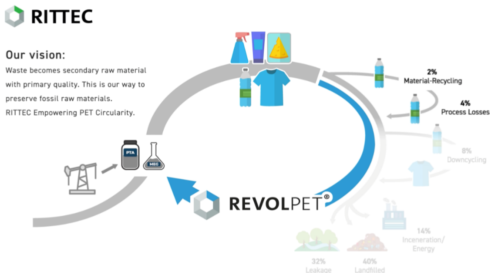
Figure 1: Realization of a circular economy for PET-containing plastics through the use of revolPET technology, which enables the recovery of the monomers terephthalic acid (PTA) and ethylene glycol (MEG) from PET in primary quality.
