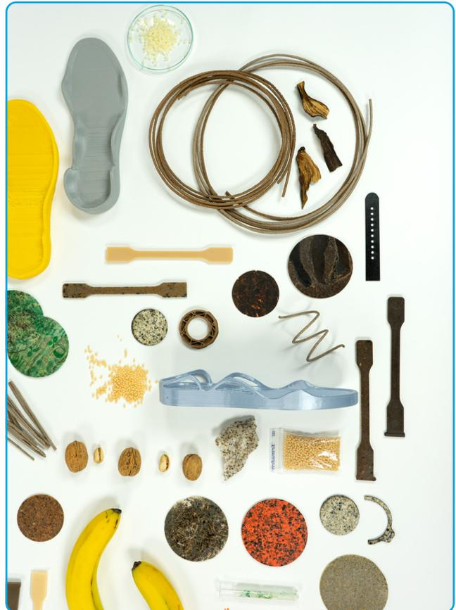
We are developing and producing bio-based and biodegradable elastic materials based on food waste such as banana peels and nut shells. They are sustainable alternatives for conventional elastic materials in various applications.
